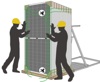
5) Cut off all the horizontal packing belts.
