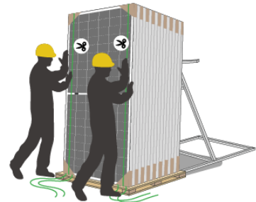
6) When there are 1-2 vertical packing belts remaining, push the module to tilt toward the auxiliary tool.
