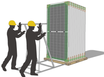
4) Place the auxiliary tool from the glass side.
